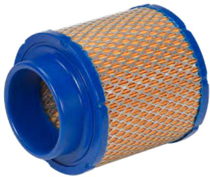
ViroSoft one-way, single-stage dry air filters are suitable for high-pulsation applications subject to a slight dust load. Typical applications include small engines (1-3 cylinders) in electricity generators, compressors, marine engines and forklift trucks, etc. This air cleaner maintains an efficiency of 99.9 % but with economical replacement cost compared to the two-stage air cleaners.
