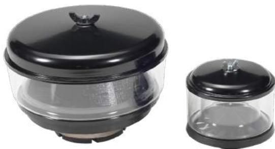
VisiClean pre-cleaner works with centrifugal force, separating off the dust particles into a dust bowl. The cyclone pre-cleaner increases the maintenance intervals for single and two-stage air filters that are used in environments with a medium to extremely heavy dust load. It additionally has the same function as a rain cap.
