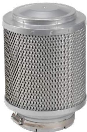
If the ViroClean air cleaners are fitted onto electronic diesel engine they must be serviced with water and washing powder every 300 hours, let it dry or use compressed air (Max 5 bar) to avoid to damage the filter element.
