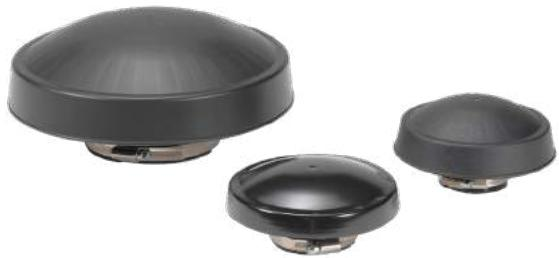
The rain cap protects the air filter against the penetration of moisture in the form of rain, snow, and splashed water and prevents bigger objects such as leaves and branches, etc. from getting into the filter, thus extending the servicing intervals. Various sizes are available in metal and plastic.
