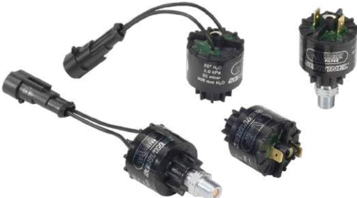
This built-in sensor monitors the degree of soiling of the air filter and emits a control signal when the predefined end-pressure differential is reached in the filter. The acoustic or optic display that is triggered alerts the operator to the filter soiling, ensuring that servicing can be carried out at the correct point in time.
